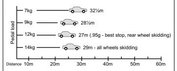
Fade test: pedal load requried for a moderate (34m/.75g) stop: 51/2kg at start of test, 81/2kg at end of test (Ideal brakes show no change)
