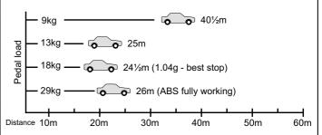
Fade test: pedal load requried for a moderate (34m/.75g) stop: 10kg at start of test, 9kg at end of test (Ideal brakes show no change) disappointing), and compared with your old Ford Escort, you'll not be complaining. However, the 323's lower speed tremors from under-bonnet, the fidgety ride over less than billiard-table main roads and an associated tendency to nibble and dither directionally as it proceeds in an ostensibly straight line, fall short of even the 121, let alone the likes of Focus
