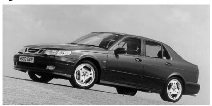
What's different? High-powered version of Saab's four-cylinder engine plus suspension tweaks equal new sporting flagship.
