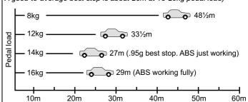
Fade test: pedal load requried for a moderate (34m/.75g) stop: 14kg at start of test, 18kg at end of test (Ideal brakes show no change)
