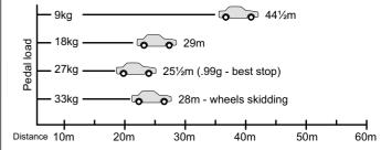
Fade test: pedal load required for a moderate (34m/.75g stop: 14kg at start of test, 14kg at end of test (Ideal brakes show no change)
