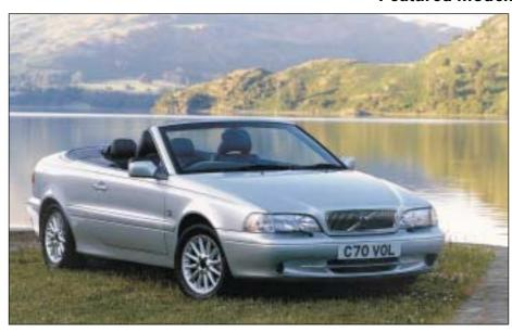
HIS VOLVO FOR ALL SEASONS IS the soft-top variant of the C70 Coupé we waxed lyrical about on its debut. But while both cars are mechanically identical, the Convertible has considerably more body stiffening, as well as a bevy of electric motors and gizmos to power the hood. The result is that it's a whopping 112kg heavier than the tin-top. It's also less aerodynamic and in this case has power-sapping automatic transmission (an £1100 extra).
